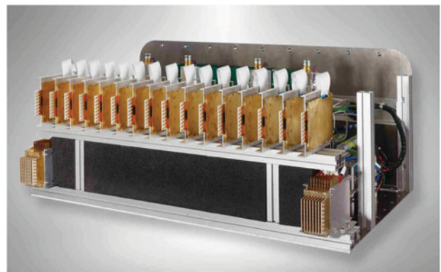
Fig. 6. MIMO array inside the frontend.
