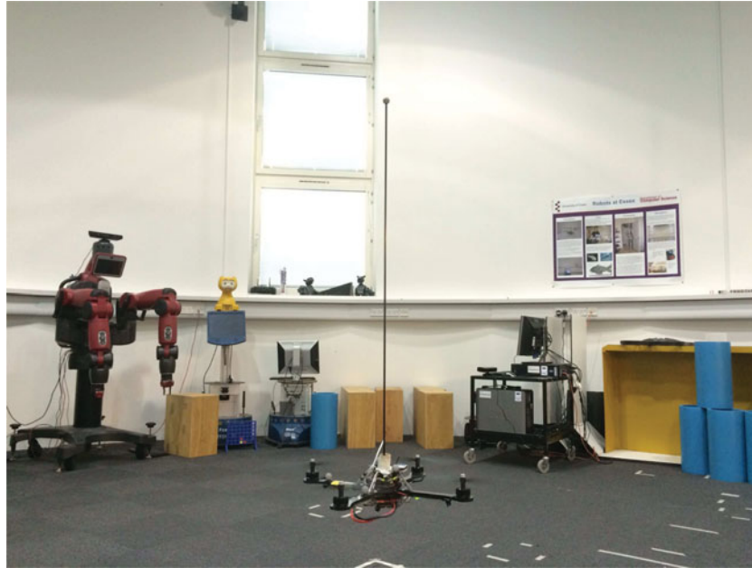
Fig. 13. An inverted pendulum on a hovering quadrotor.
