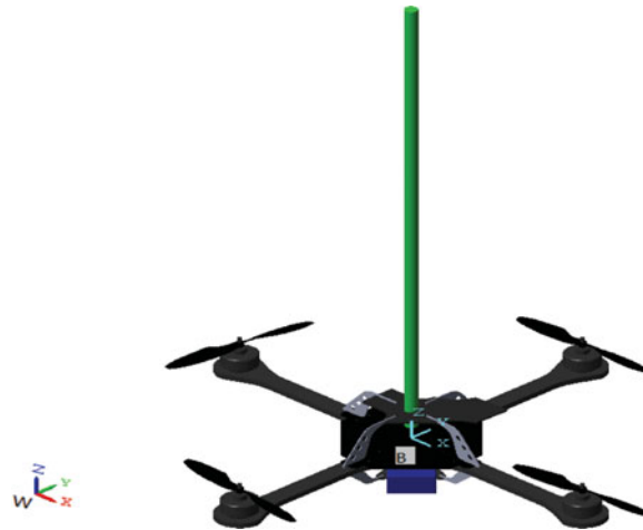
Fig. 1. Fixed body and world coordinate systems.
