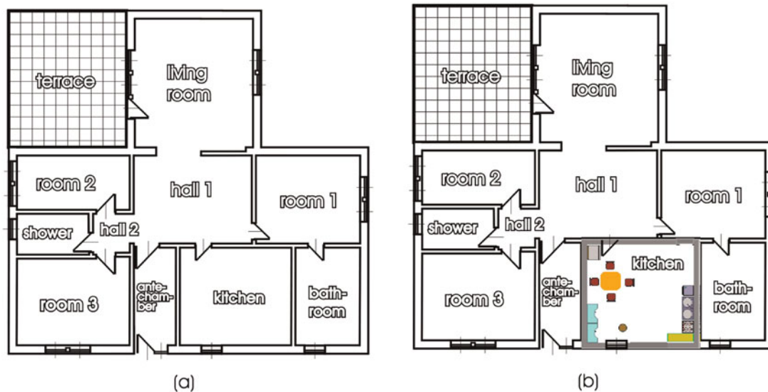
Fig. 10. (a) A floor layout corresponding to the hypergraph from Figure 9 and (b) a floor layout with a kitchen arrangement. [A color version of this figure can be viewed online at www.journals.cambridge.org ]
