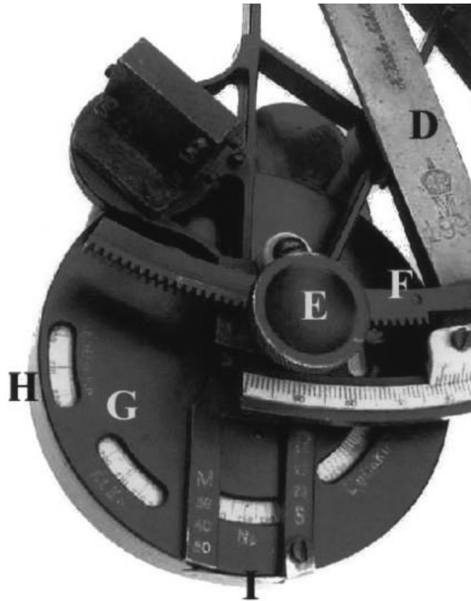
Figure 2. The distance scales of the Haecke rangefinder. G is a rotatable drum 3\frac{1}{2} inches in diameter, \frac{5}{8} inches deep. The knob E rotates a disc inside the drum as the index system is adjusted to align the sight. The disc is printed with six concentric scales of distance in metres. The three outermost scales relate to the masthead height of three different classes of ships while the three innermost scales relate to the funnel height of the three classes of ships. See Table 1. The drum G can be rotated to align one of the six windows H over the appropriate scale depending on which class of ship is being observed and whether the masthead or the funnel is being used. The M and S scales at I give masthead height and funnel height in metres for the three classes of ships. The scales at I also could be used to measure distance to any other object whose height happens to be the same as that of the masthead or funnel of a ship. A detent at I assures precise alignment of the index mark in the window with the scale. See Table 1 for translation of the abbreviations marked on the scales.
