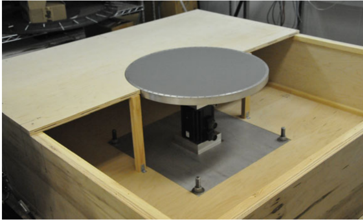
FIGURE 26. (Colour online) Photograph of the rotating disk system with the low-pressure enclosure partially open.
