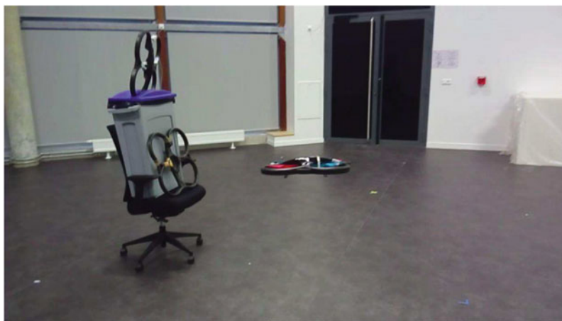
Fig. 11. Obstacle avoidance experiment. Note that the obstacle has an irregular form and the vision algorithm is capable of detecting it.
