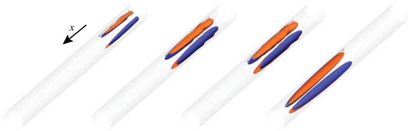
FIGURE 7. Linear optimal solution for Ma = 0.80 at solution times t = \{0, 3, 4.5, 15\} . Isosurfaces of the streamwise perturbation component, u'_1 = 0.60 \times \max(u'_1) (red) and u'_1 = -0.60 \times \max(u'_1) (blue).
