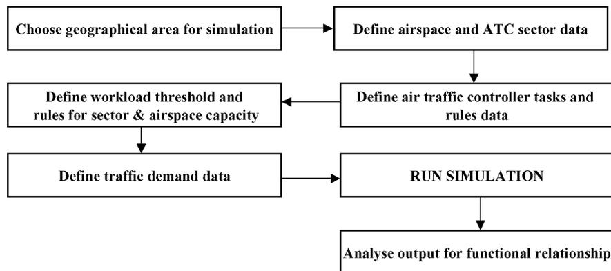
Figure 4. A scheme for estimating airspace capacity.
