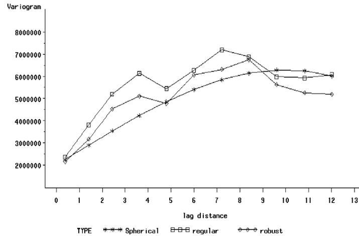
Figure 8. Covariogram of current traffic data for the ATC sectors of Europe compared with a theoretical spherical covariogram.
