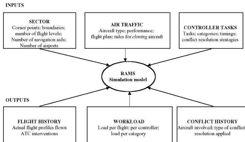
Figure 3. The inputs and outputs into the RAMS model.
