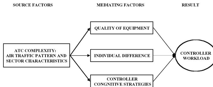
Figure 1. Factors affecting controller workload.
