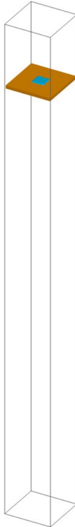
FIGURE 13. (Colour online) Schematic representation of the simulation set-up showing a single pore filled by the liquid (blue). Injection of the liquid through the single pore is modelled by imposing a liquid flux boundary condition on the top surface of the pore using an exponential slowing injection speed obtained from experiments.
