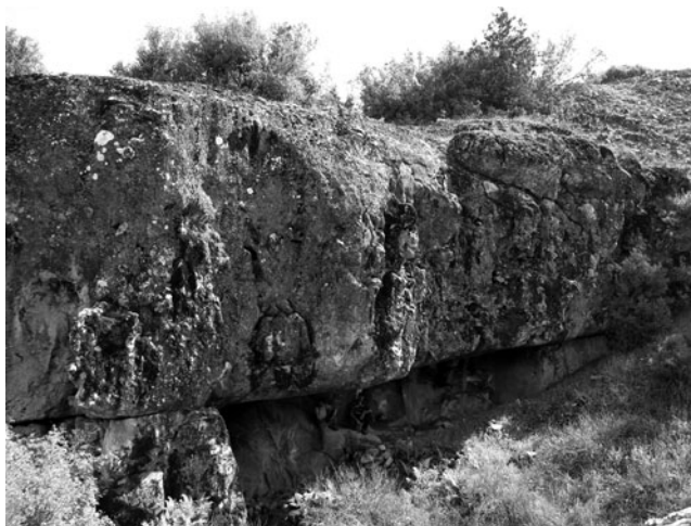
Fig. 6. View of the underground quarry 3C, district 3, at Göktepe showing the thick breccia layer above the white marble vein. (Photograph by the authors.)
