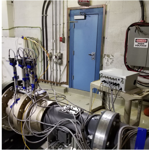
Figure 10. Rotary and linear traverse systems.
