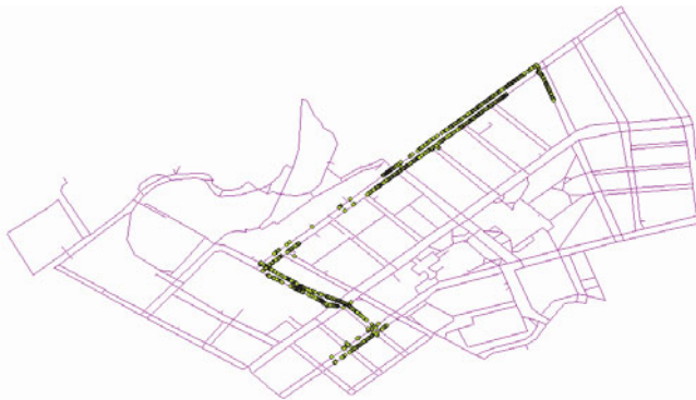
10b. Projected result data to the matched sidewalk segments on campus sidewalk map.
