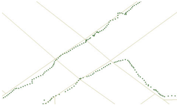
Figure 4. An example of GPS points overlaid on sidewalks on campus.
