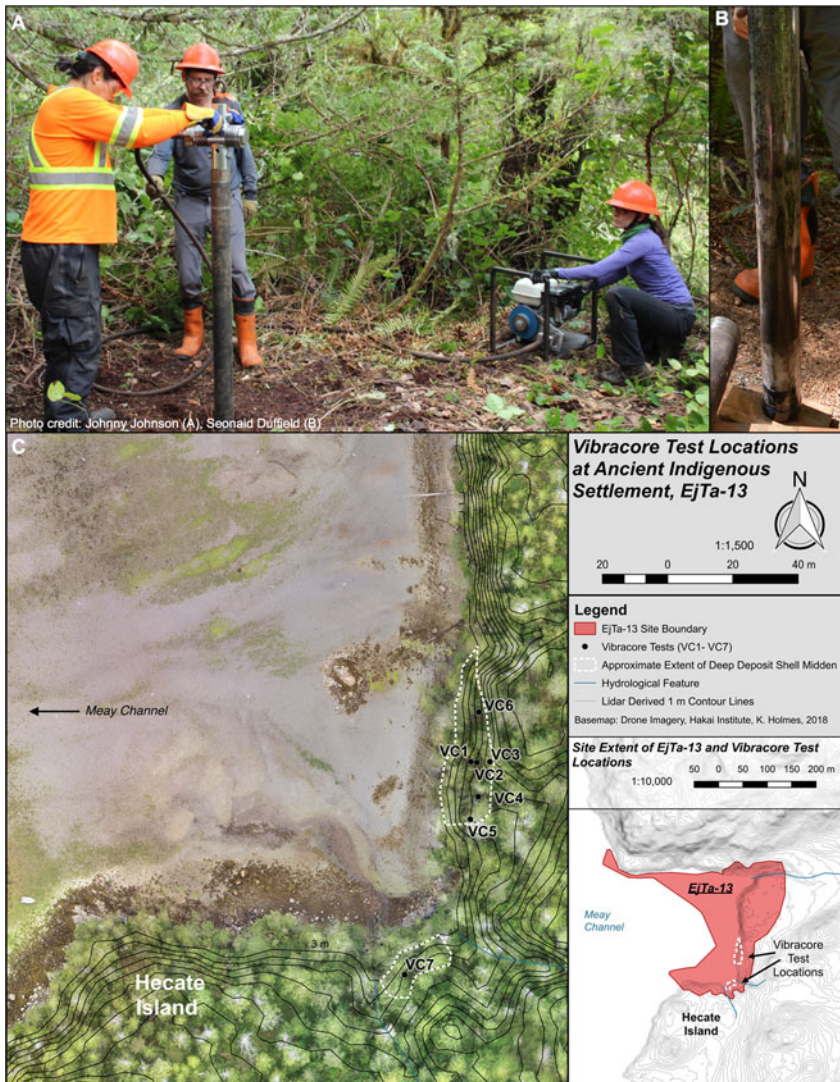
Figure 2. (A) Maxwell Johnson Jr. (Heiltsuk community member) operating the vibracore, while archaeologist John Maxwell directs the “flexcable,” which feeds rotational power from the motor to the drill head, and Seonaid Duffield operates the motor (photo courtesy of Johnny Johnson, Wuikinuxv Nation); (B) an example of a vibracore sample tube containing a sediment sample (photo courtesy of Seonaid Duffield); (C) map of test locations at EjTa-13 (created by Seonaid Duffield).
