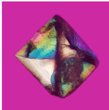
Fig. 3. Kingsgateite crystal showing anomalous birefringence. The image is looking down the c axis under crossed polars with the crystal 45^\circ from the extinction position and the gypsum (first-order red) plate inserted with its slow direction oriented NE–SW.
