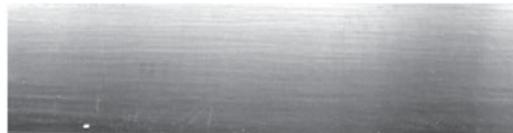
FIGURE 6. Snapshot of the lengthwise streaks at the pre-growing stage at  $x = 220$  cm (image size approximately 30 by 10 cm<sup>2</sup>).
