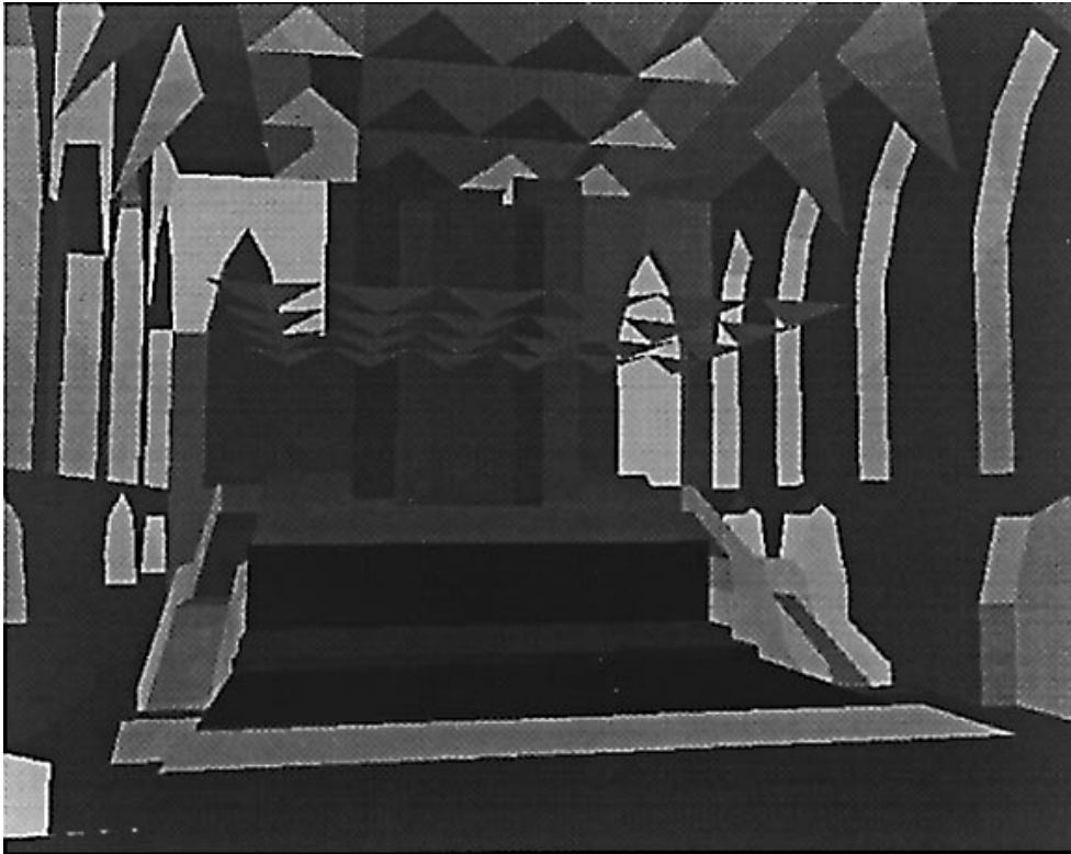
Figure 2. Example of realtime visual rendering (local illumination with flat shading and without textures).
