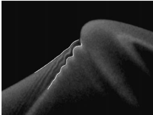
FIGURE 13. Sample digitized image with computed capillary wave profile and corresponding image of toe edge highlighted by white pixels.
