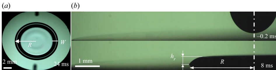
Figure 2. Snapshots of the dynamic spin-coating process obtained from (a) camera 1 and (b) camera 2, with an ethanol drop of 1.13 mm in radius and the rotating speed being 3000 rpm.
