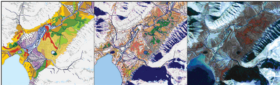
Fig. 11. Map subsections - Gipsdalen valley. The conventional map is displayed to the left, the satellite based map in the middle and a 3-band Landsat image (ch421) to the right.
