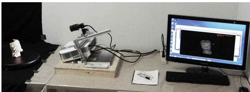
Figure 3. The set-up of the pilot project structured light system in the Larnaka District Museum study room.
