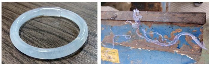
Silicone grease encapsulated tube, before and after testing
