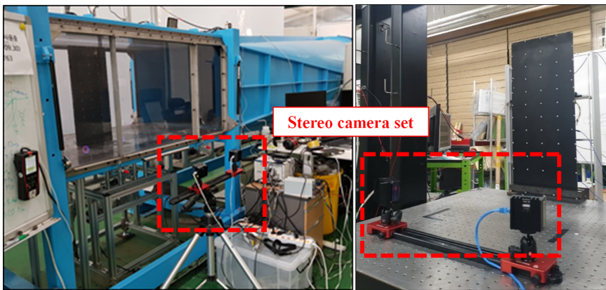
Figure 21. Stereo camera set-up for deformation shape measurement; in wind-tunnel (left), EFT (right).
