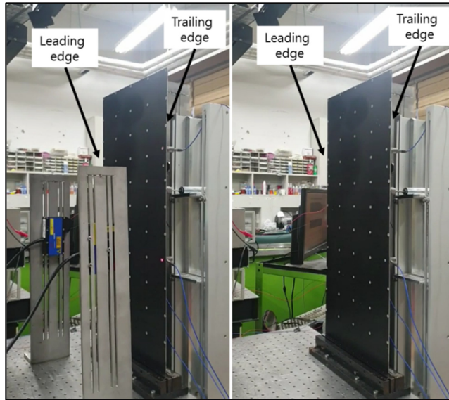
Figure 18. EFT test set-up by LDS(left), and Accelerometer (right).
