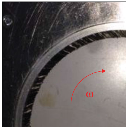
Figure 7. (Colour online) Formation of a brush seal lay angle.
