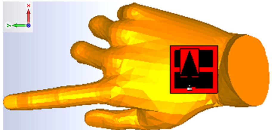
Fig. 2. The integrated design flat layout against the SAM human hand model.
