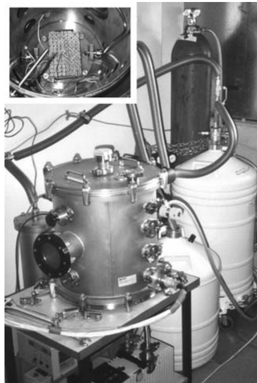
Fig. 1. Mars simulation chamber at the Space Research Institute of the Austrian Academy of Science, Graz. The chamber (foreground) is cooled by a liquid nitrogen circuit. In the white containers behind the chamber the liquid nitrogen is stored; it is driven through copper tubes by the pressure that is provided by gaseous nitrogen from the tank visible in the background; the chamber atmosphere is produced from gaseous \text{N}_2 and \text{CO}_2 . Inset: chamber without a lid, containing a rack with 96 samples in small plastic tubes.
