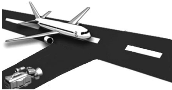
Figure 2. Illustration of where a camera is located during an aircraft's landing or takeoff to capture its 2D projection image.
