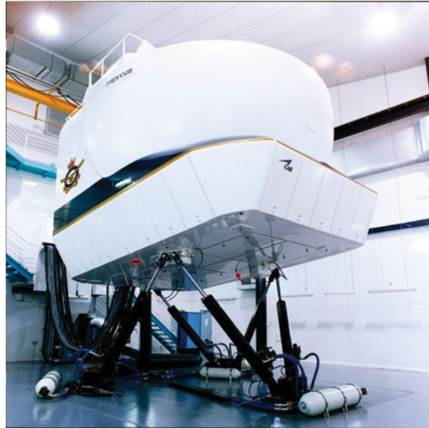
Fig. 1. CAE's version of the Gough–Stewart motion platform for a flight simulator.
