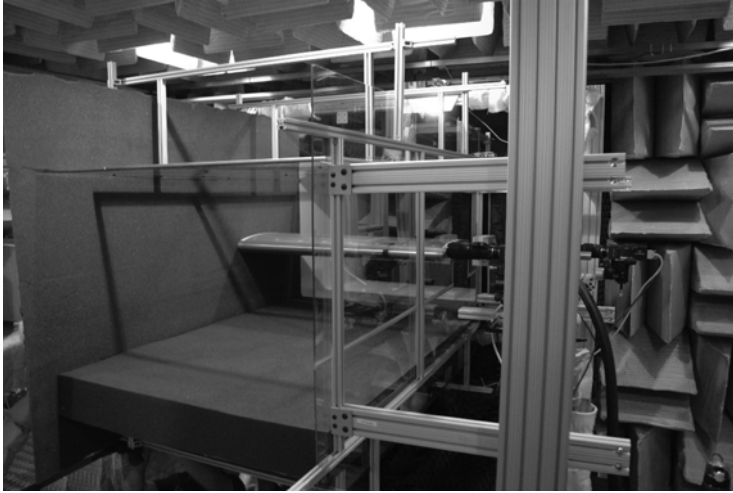
FIGURE 13. Photograph of closed-wall test section for PIV measurements. The foam ceiling and one foam wall are replaced with clear polycarbonate panels.
