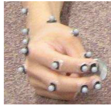
Fig. 3. (Colour online) A subject with auto reflective markers attached to the finger joints holding a small object (coin).
