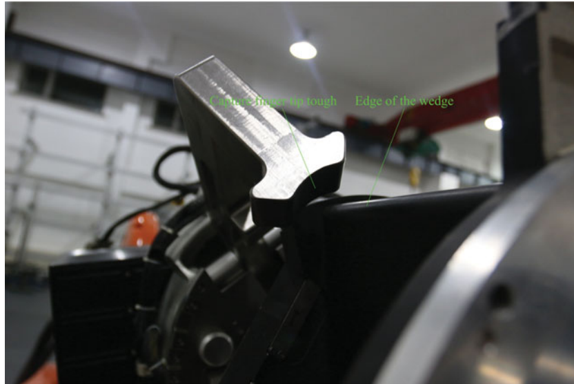
Fig. 21. Interference failure capture.
