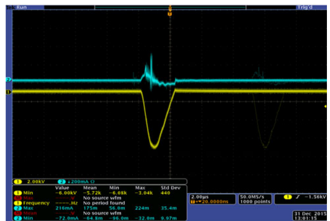
Fig. 9. Oscilloscope current-voltage trace of the cold plasma jet at 6 kV/25 kHz.
