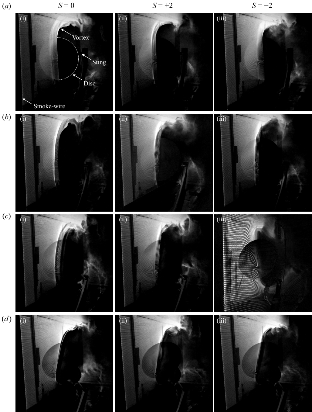
Figure 4. Streakline patterns over the disc at an oblique downstream viewing angle. Re = 2.7 \times 10^4 , S = 0 and \pm 2 , and (a–d) \alpha = 0, 12, 24 and 36^\circ . The image in panel (ai) ( \alpha = 0 and S = 0 ) is annotated to aid visualization. Coherent vortical structures form at the pressure side, upstream surface, of the disc and cyclically shed into the wake region. The images shown here correspond to frames where vortical structures are aligned with the disc’s central axis, prior to being shed into the wake region. The reader is encouraged to watch Movie 2 and Movie 4 to develop familiarity for the viewing angle in which the flow fields are captured here.
