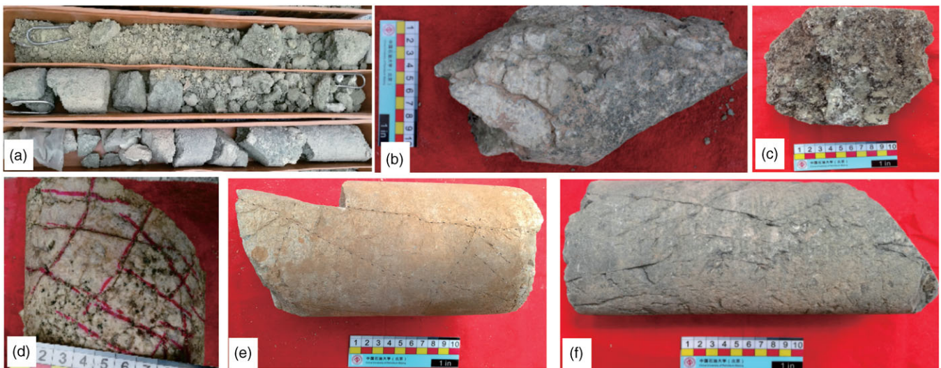
Fig. 4. (Colour online) Images of different weathered granite reservoir cores taken from wells. (a) Regolith, greyish white, gritty, weathered granite, original structure destroyed by weathering (Well S87, 1070–1080 m). (b) Regolith, dark-grey massive coarse-grained granite with traces of weathered remains (Well S6, 1078.2 m). (c) Regolith, remaining oil spots (Well LGX601, 3094 m). (d) Dissolution zone, flesh-red quartz feldspar sandstone, development of articular cracks and dissolved pores (Well Z362, 1219.4 m). (e) Fracture zone, greyish-white medium-grained granite, two groups of cracks with different angles (Well S18, 1185 m). (f) Fracture zone, grey blocky granite and reticulated multiple groups of cracks (Well S133, 1384.6 m).
