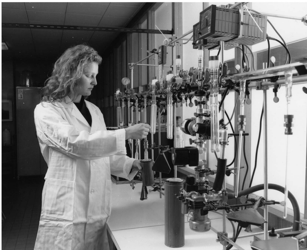
Figure 3 First preparation line for AMS targets at the Royal Institute for Cultural Heritage (KIK-IRPA) (1989, © KIK-IRPA)
