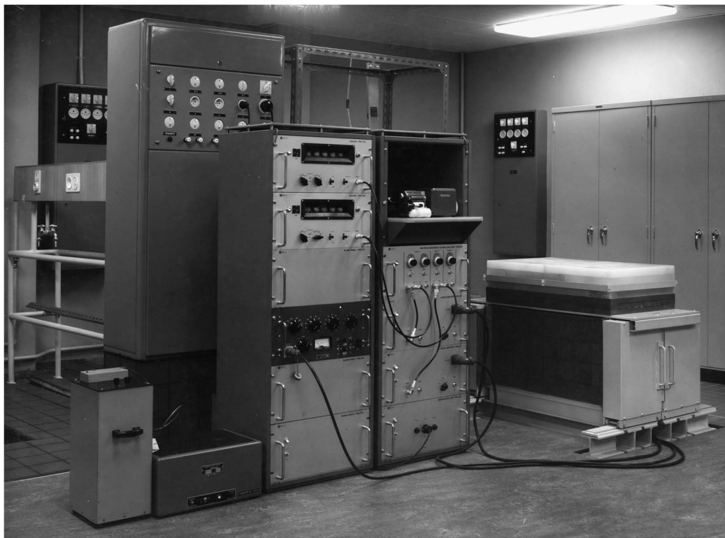
Figure 2 Proportional gas counter at the Royal Institute for Cultural Heritage (KIK-IRPA) made by the Belgian company M.B.L.E. (Manufacture belge de Lampes et d'Électronique) – before 1978 (© KIKIRPA).
