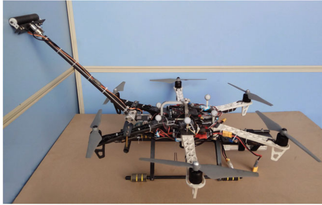
Figure 4. AM system structure.
