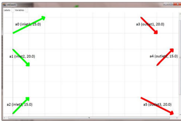
Fig. 2. A seed graph with three inlets and outlets.
