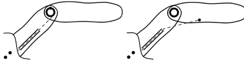
Fig. 3. Wire actuation with (left) and without (right) access to the joint.
