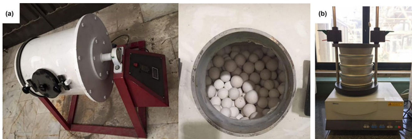
Fig. 3. (a) The ball mill and (b) the vibration sieve shaker for preparing the raw bentonite samples.
