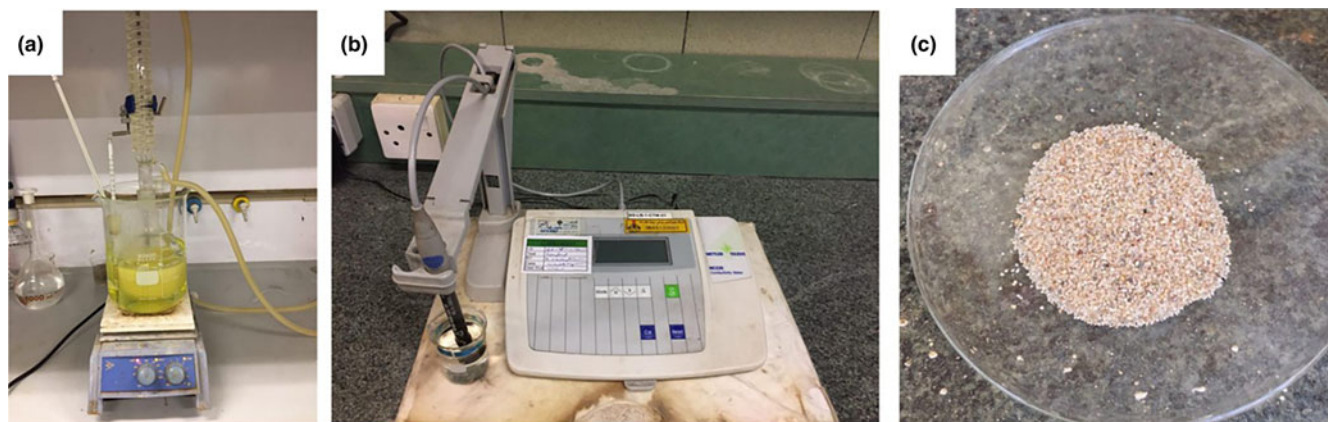
Fig. 5. (a) Preparation setup of the activated clays. (b) Device for measuring the conductivity of distilled water. (c) Acid-activated clay after drying.
