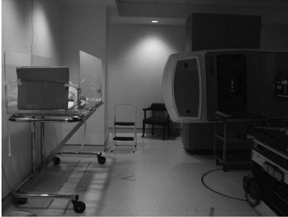
Figure 4. Standardized rotations of 90^\circ and 45^\circ for gantry and collimator, respectively, and a maximum field size ( 40\text{ cm} \times 40\text{ cm} ) at extended distance during treatment.
