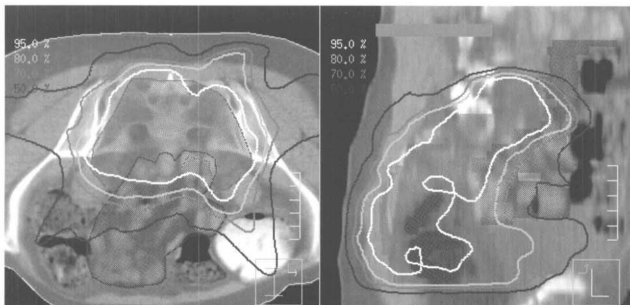
Figure 3a. Transversal and sagittal view of a dose distribution of an IMRT plan as calculated with method 1 as prescribed in this paper after recalculation of the dose distribution in Pinnacle. The 95%, 80%, 70% and 50% isodose lines are displayed.
