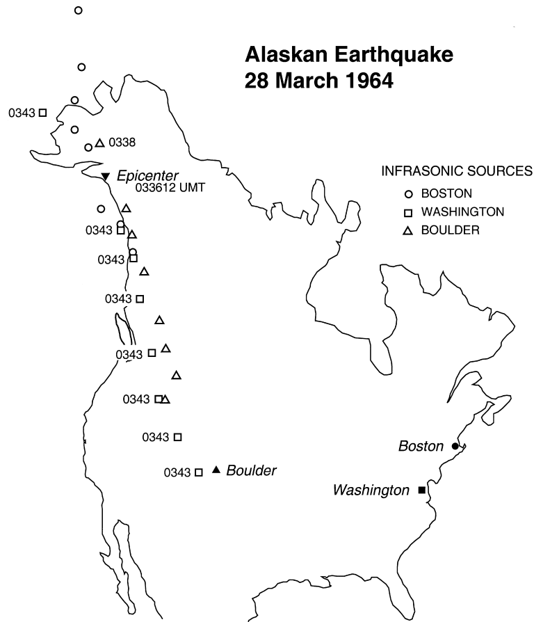
Figure 1. Calculated positions and times of seismic-to-air wave conversions after the Alaskan earthquake of 28 March 1964 (after Figure 6 of Young and Greene, 1982).
