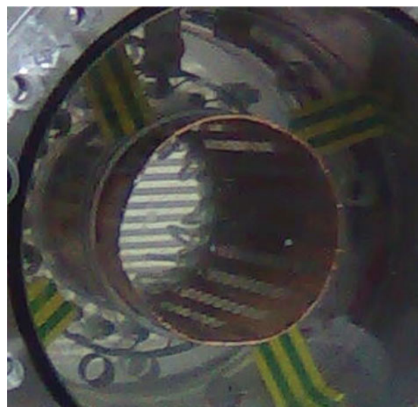
Fig. 11. (Color online) The cylindrical flashboard plasma source demonstrates that the circuit board material is easily rolled into a 7.6 cm-diameter cylinder. The chains of copper pads are visible running axially along the inner surface of the rolled cylinder.
