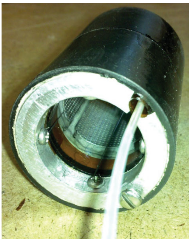
Fig. 7. (Color online) The compact ferroelectric plasma source is only 3.8 cm in diameter in order to fit inside the bore of the 8 T solenoid. The high-voltage lead must be well-insulated and it connects to the metalized outer surface of the ceramic cylinder through a hole in the aluminum ring.
