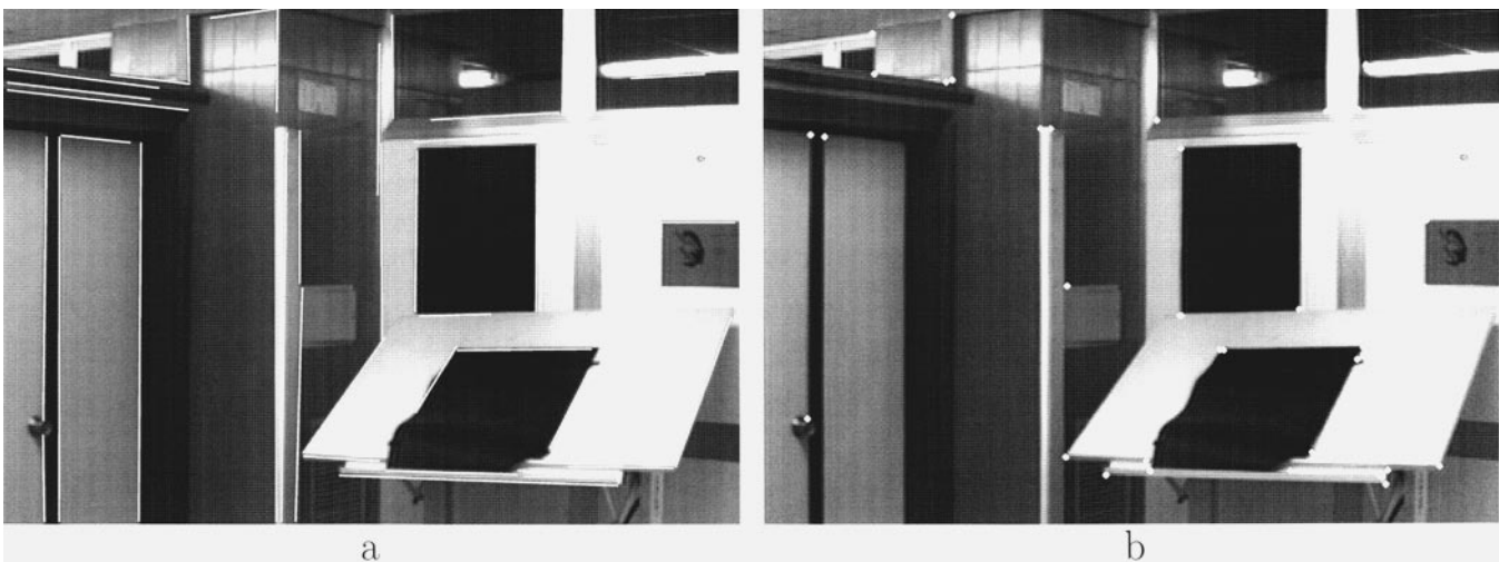
Fig. 1. a.-Image of the laboratory with the lines extracted (filtered in gradient and length ). b.-Characteristic points selected along the lines.
