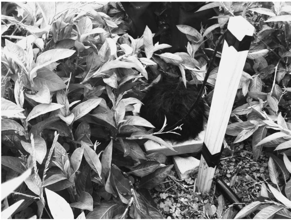
Figure 6. The field recorders sat on wooden bases and were built using Rycote zeppelin end caps and synthetic fur to protect the mics against rain and distortion created by high winds.
