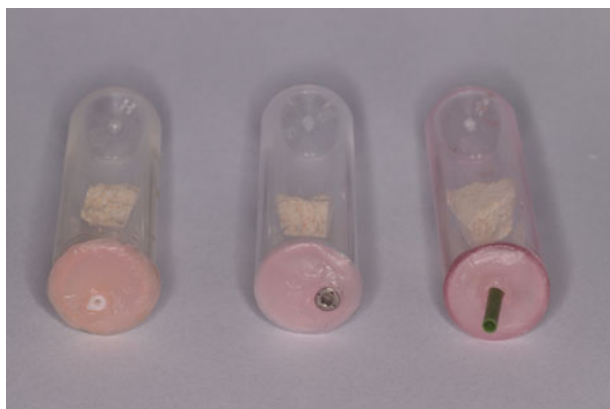
Fig. 1. The middle-ear model with Shepard, titanium and T-tube grommets embedded through dental wax. The effervescent solid can be seen in the tube.
