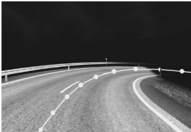
Figure 11. ALC controlled by high precision GPS in combination with the road database on a hilly and curvy road in the driving simulation.
