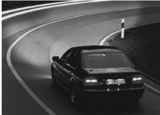
Figure 9. Adaptive Light Control.
