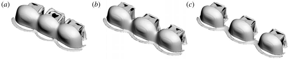
FIGURE 9. Isosurface contours of the vorticity around three parallel-aligned cubes for different gap distances: (a)  $G = 0.5h$ ; (b)  $G = 1.0h$ ; and (c)  $G = 1.5h$ .
