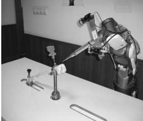
Fig. 4. A physical setup. Two CCD cameras are rigidly mounted on the end-effector of an Motoman Robot for performing hand–eye calibration.
