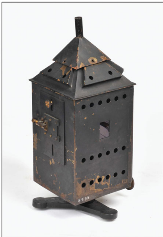
Fig. 6. A petroleum-burning lamp used to create beams of light for the variometers. The lamp featured a series of adjustments to optimise its use, including colour filters, a micrometrically adjustable slit, and position controls. Photograph: Museum of Science and Technology, Oslo, Norway.
