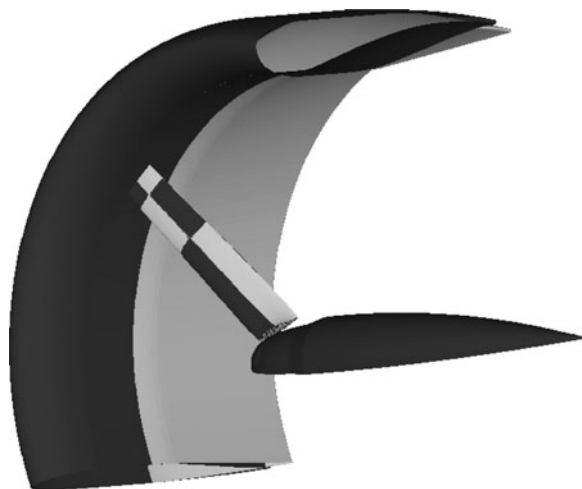
Figure 23. Comparison of baseline (light gray) and optimised (dark gray) blade and duct surfaces.
