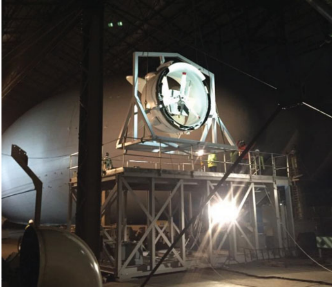
Figure 3. (Colour online) Propulsor test rig (Source Hybrid Air Vehicles Ltd ).
